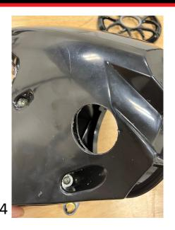
On the inside you will need to cut or grind down the material in area of the hole.
