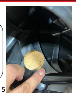
Once you remove the material you can test fit the speaker.
