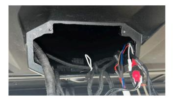
Before proceeding with the installation of the WWX-USB3.5, ensure that you have proper clearance for its body at the chosen location. Once the location is determined, proceed to drill a 1" hole, allowing you to easily feed the cabling through the opening.
