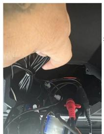
Secure the cables' slack with zip-ties and tuck them towards the back left-hand side. To prevent any rattling, you can wrap the cable bundle in felt tape.
