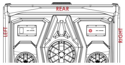
Expandable Amplifier Slot: The plate can be replaced with Wet Sounds AR-AMP 2CH. The AR-5 Defender Max comes pre-wired to accept the AR-AMP 2CH for easy installation. A DT connection is included in the AR-5 wiring harness to wire additional speakers and RGB lighting.
