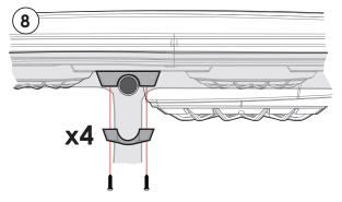
Attach the (4) center clamps with the (8) M5 screws provided to secure the roof to the center roof rail.
