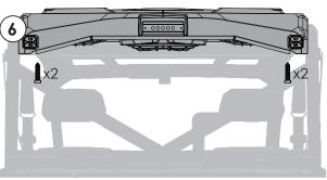
Fasten the back of the roof with the (4) M8 torx screws provided.
