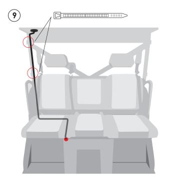
Secure the wiring harness to the post by using (2) zip ties near the locations marked above.
