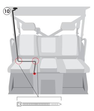
Wire the harness towards the battery (located under rear seat behind panel) and secure it to avoid it touching hot or moving parts. Extra (2) zip ties are included if needed.
