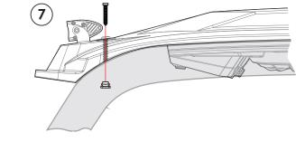
Use (3) M6 torx screws and (3) M6 flange locknuts to fasten the front of the roof. Do not overtighten the screws.
