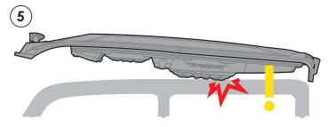
Be careful not to bump the speaker grilles while lifting the roof over the rails.
