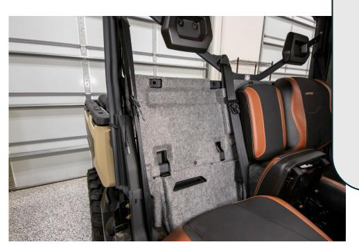
With the back seat removed now to remove the carpet panel in order to route the harness. Once routed under the seat you can now place the carpet panel back and connect the positive and negative to the battery.
