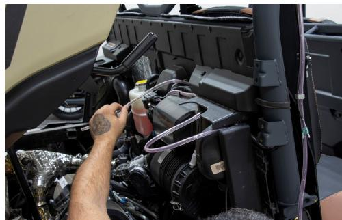
On the opposite side similar location fish wire through the side rail and tape to your tube and the wire that triggers it to spray this will be extending later. You will see similar tubes routed just follow that path to make it back to the OEM location. Once you have that routed back to the OEM location you can now put the AR-Roof on.
