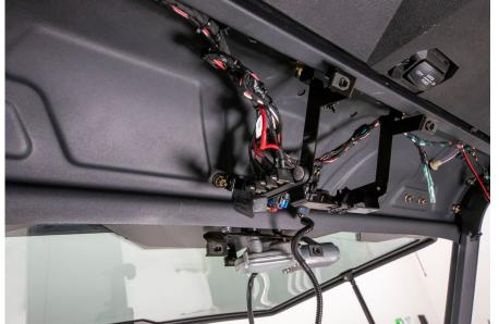
With the main harness you will want to remove the loom from it in-order to better arrange it in the area. We recommend taping the harness up to keep it organized and locate the plugs for the doors on the corresponding sides
