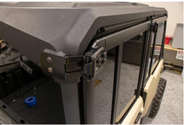
With the hinges now mounted you can put the back window back on and you are now finished with the installation of your new AR-Defender Roof!!
