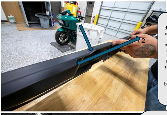
On the front panel with dummy switches notice where the arrows are pointing. You will need to trim the front portion of the panel down to the line where the arrow is pointing and between the area where the second arrow indicates.
