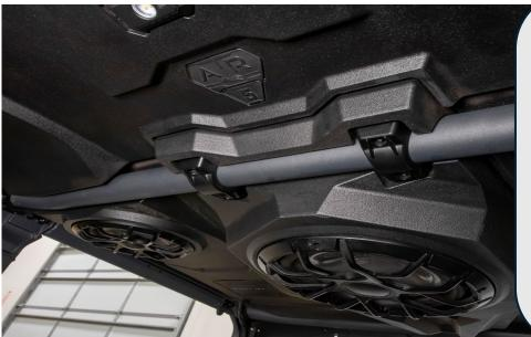
Now you can move to the middle of the roof and start placing the clamp mounts in place 4 total. Then time to remove the rear seat on passenger side to route the main harness to the battery.
