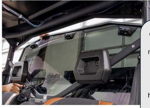
Once the back glass is removed you can now remove the front part of the roof then the back part. That will leave you with the power window harness up front. You will want to remove the hose for the windshield fluid and the harness that goes along with it. we will need to re-route them on the other side of the defender.
