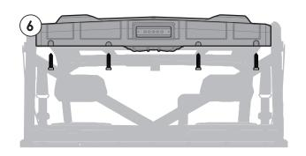
Fasten the back of the roof with the (4) M6 torx screws provided.
