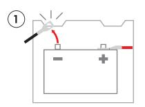
For safety reasons, we recommend disconnecting the battery before starting the installation.
