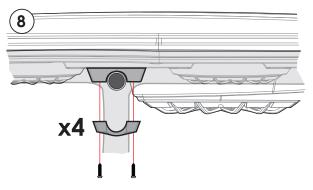
Attach the (4) center clamps with the (8) M5 screws provided to secure the roof to the center roof rail.
