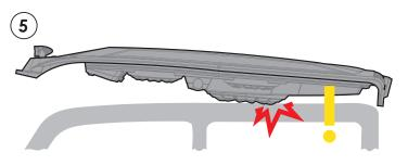
Be careful not to bump the speaker grilles while lifting the roof over the rails.
