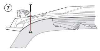
Use (2) M6 torx screws and (2) M6 flange locknuts to fasten the front of the roof. Do not overtighten the screws.
