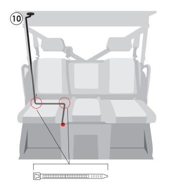
Wire the harness towards the battery and secure it to avoid it touching hot or moving parts. Extra (2) zip ties are included if needed.
