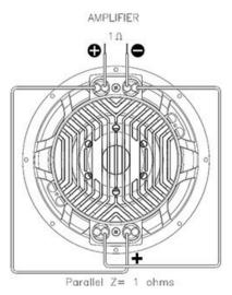
REVO XXX Subwoofers are available in Dual 2 Ohm Impedance only. This means that each subwoofer can be wired for a total impedance of either 4 Ohm (with the 2 voice coils wired is series) or 1 Ohm (with the 2 voice coils wired in parallel).
