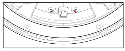
Note: ZERO Series has a standard Deutsch connector compatible connection. (PN: DT04-2P) PIN 1 (+) PIN 2 (-)
