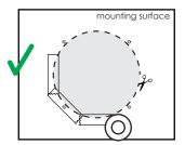
For speaker alignment, the terminal indicates the bottom of the speaker, and the opposing lock tabs help for horizontal alignment.
