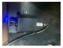
Mount the control just shy of the glove box you can and pop 2 holes big enough for the AUX cable to fit through.
