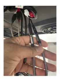
Plug in your 3.5 Aux cables and tape/heat shrink and rout them towards the back of the roof with a Long zip Tie or a wire grabber. removing the Secondary amp will make things easier to fish the cables through.
