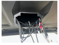
Once you have the box secured then time to wire into the MC-2's harness. Wire up Blue to Blue and then extend your power and ground to go towards the back with the Aux Cables.
