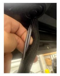
With the amp out you will pull the grommet out some and will need to cut the electrical tape in order to slide the cables into the main harness of the roof. You will tuck the cables in till you get down to the area were its connected to the battery.
