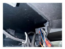
Wipe area with alcohol let dry then apply double side tape to the Talk Back Mic. mount the unit on the left-hand side add some foam padding to prevent rattle.
