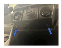
Under the switch panel you will locate 2 tabs to be removed.
