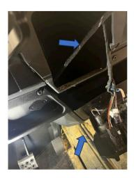
Route your cable along side of OEM harness and up into the dash area. In order to make your way to the glove box. Any access wire you can tie up in this area.
