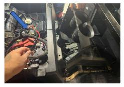
Wrapp the aux cables in tesa tape to make the run easier. There are a few tabs you will need to remove from the cupholder panel. This will allow you to run the cables up front following OEM wires.
