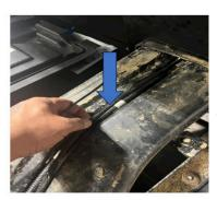
Once the rear center console is removed you can run the Aux cables along side OEM wire.
