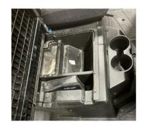
Lift passenger sear and remove tray to gain access and pull the AUX cable from the back.
