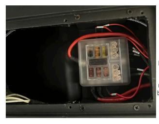
The Fuse box is in the same area as the secondary amp. There is a 12v output location available. remove cover and place a 2amp fuse in the empty location. And connect your red wire from the talk back mic and ground at any ground post.
