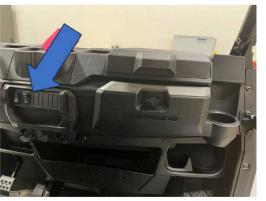
The center switch panel will need to be removed to gain access to the glove box.
