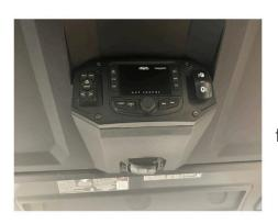
You will need to remove 4 Allen screws to gain access behind the radio. You will have room on both sides of the MC-2.
