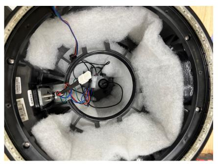
Unplug the 2pin adapter that's connected to the driver
