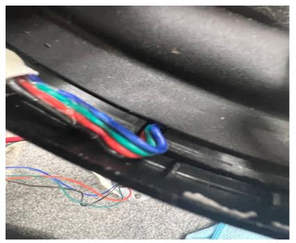
The RGB wire sits in a notch in the housing that lines up with the notch on the mid bass. Once you line them up your led wire will pass through. Make sure to note where the notch is for the RGB wire to pass through. Make sure when removing and installing that the wire is situated correctly.
