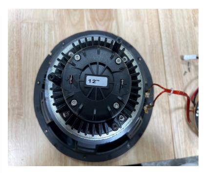
The HLCD is mounted to a plate that is screwed on to the back of the REV12 Mid bass driver with (4) hex screws you will need a 4mm hex driver. Once the Cross over is removed you then will see the HLCD that houses the Diaphragm. There are (4) 3mm Allen screws that hold the cover on.
